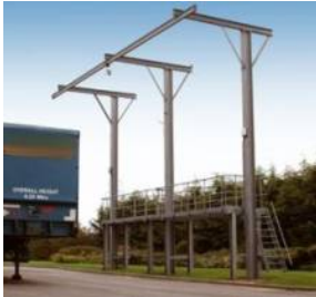
Most sheeting platforms are simple drive-through systems providing a guardrailed platform on each side of the vehicle(Fig. 8)
