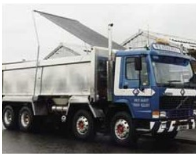
unrolling sheeting from front to back of the vehicle body (Fig.1)
