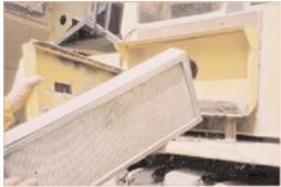
Regular maintenance of the systems is essential and the cabs cleaned regularly with vacuum systems.
