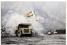
The cabs should be fitted with filters appropriate to the risk created by the dust.
