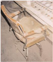
Areas of spillage such as around bagging plants should be kept clean and vacuumed regularly. Never use a brush as it makes dust airborne.
